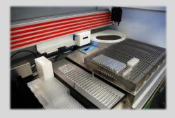
Available with 2 or 4 pipetting probes, GC Processor is a suitable solution for medium labs requiring a safe and fast processor hosting 80 samples and 120 gel cards in 112 cm long platform.
