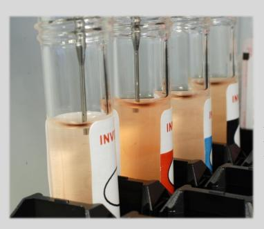
Samples are sourced from primary tubes through predilution performed in deep well tubes or standard microtiter plate format.
